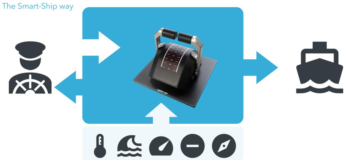
In the next step we link any kind of sensor data to the lever and provide the operator with real-time crucial operational and dynamic feedback through a force, vibration, resistance or detent. This changes the system from feed-forward to a two-channel feedback system.
