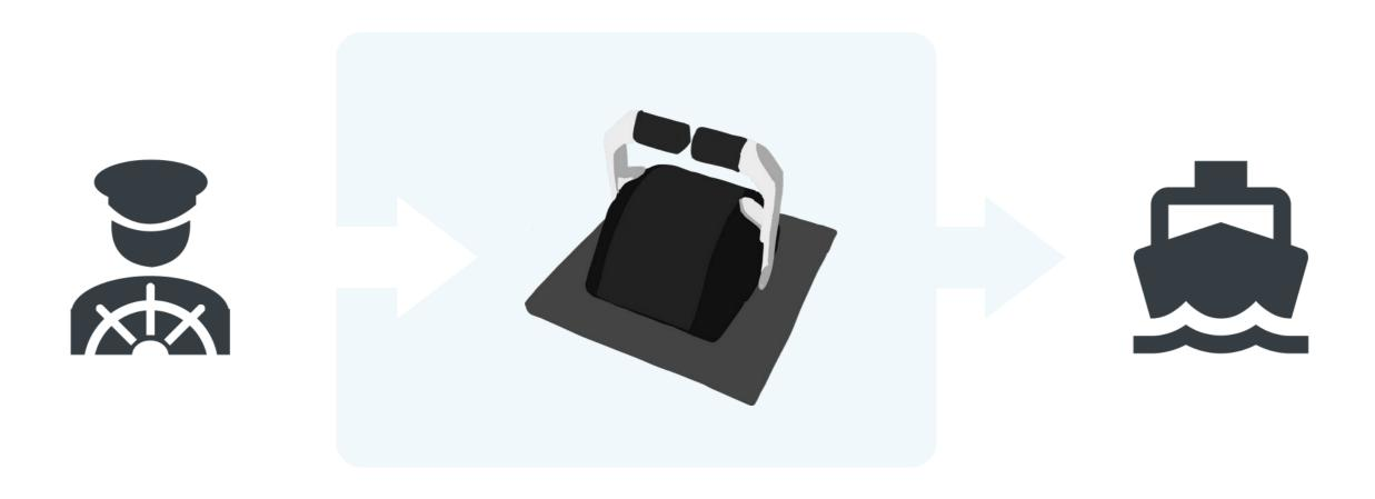
In the traditional situation, the operator will give an impulse to a control lever upon which the control then converts this impulse to an action in the vessel (engine, rudder etc.)
